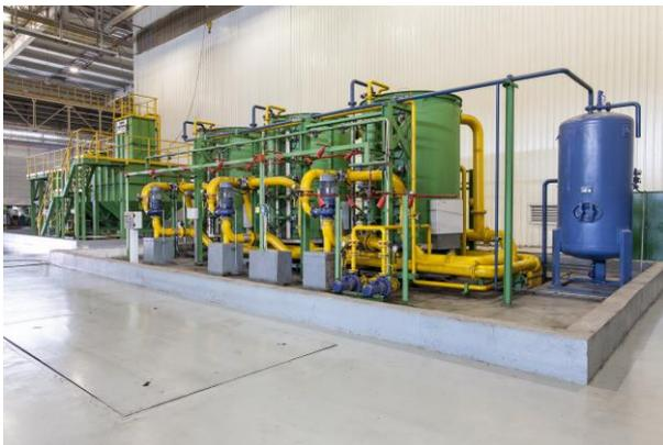
Example of a rolling-oil treatment plant using a SUPAFINE<sup>®</sup> filter system.
