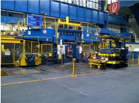
Ready for new tasks: the SMS 20-roll cold rolling mill at Outokumpu Nirosta GmbH Krefeld.
