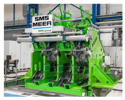
Quingdao is to receive a 3-roll precision sizing block, Type PSM 380/5, from SMS. The photo shows a PSM in the SMS workshops in Mönchengladbach.
