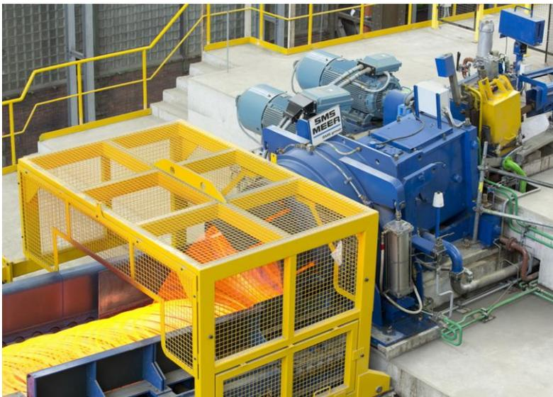
Loop laying head in a wire rod line. One of these will be installed in Saarstahl's new wire rod delivery section.
